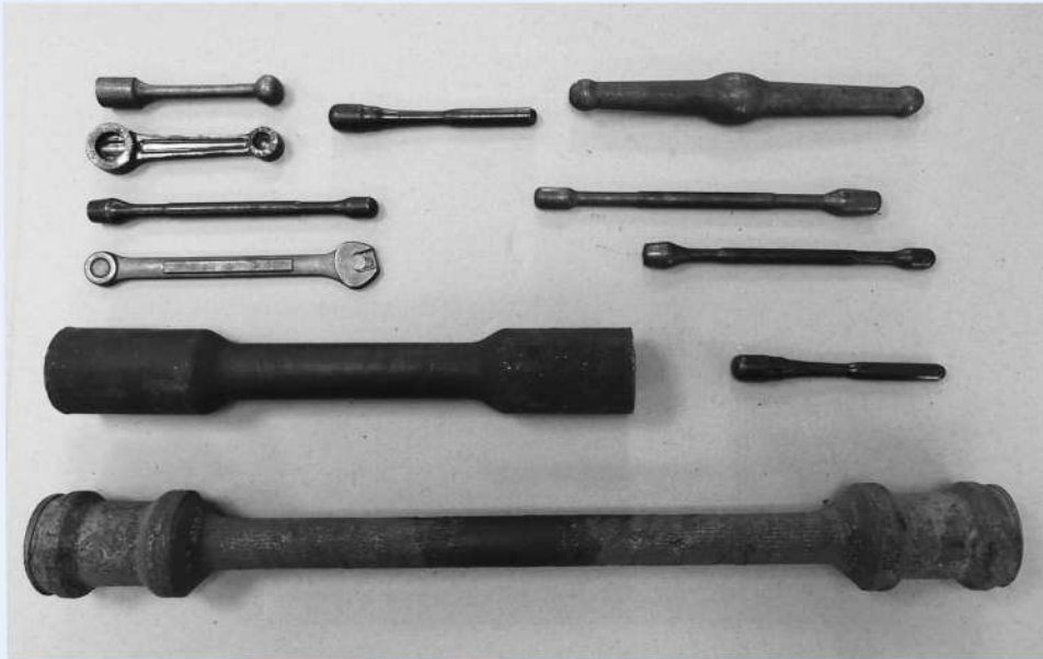
ROLLING PREFORMS FOR SUBSEQUENT FORGING
