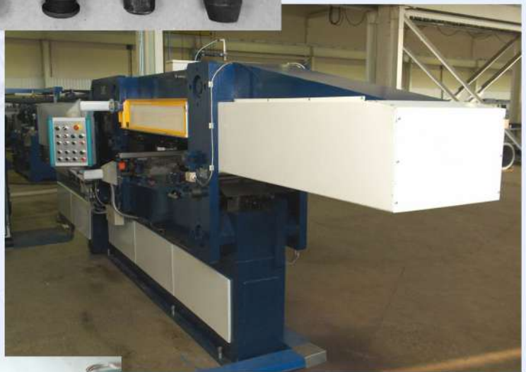
CROSS WEDGE ROLLING LINE WRL4014TS
